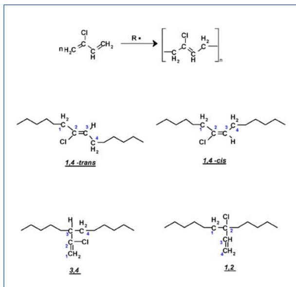
Figure 2- Basic polymerization scheme
